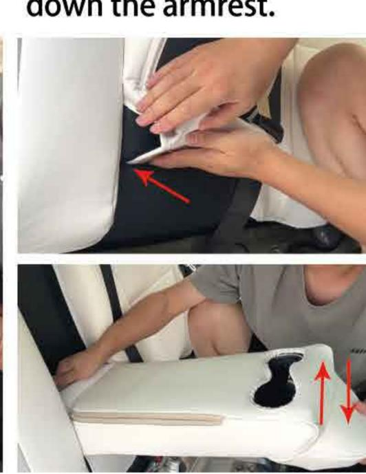
16. Insert this part from here. Swing the armrest box up and down, and pull back. out this part.
