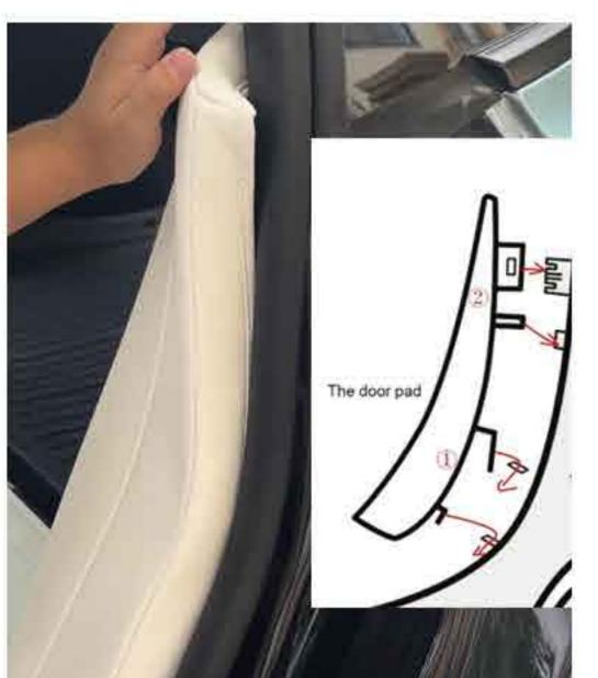
22. Then it will be installed against the snap back to the original position.
