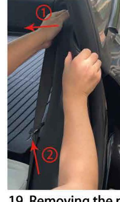
1) Pull out the upper part of the door pad 2 Lift the door pad up 19. Removing the piece requires a bit of skill. Start by pushing it towards the inside of the car, then pull it towards the front of
