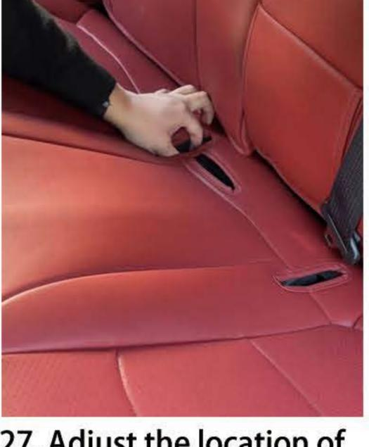
27. Adjust the location of back to its original position. suitable position. Pull out the seat belt socket.
