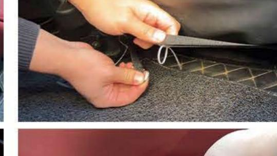
12. Use the mental hook to join the two strips together ((both front and back).
