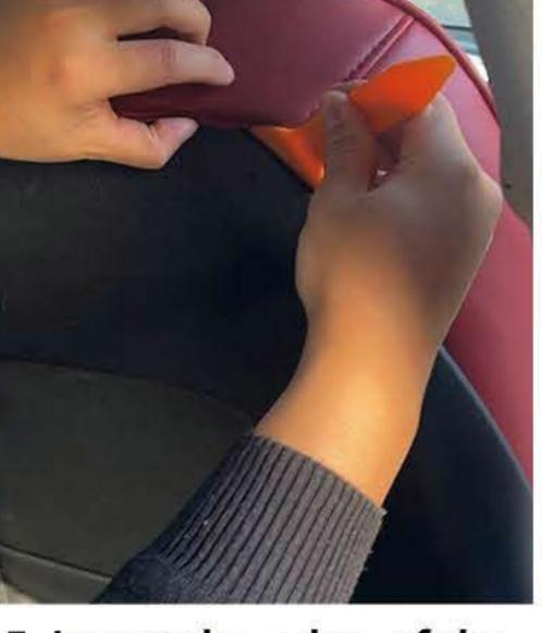
15. Insert the edge of the seat sleeve into the gap.
