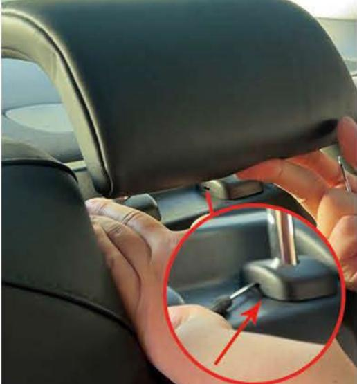
3. Pull up the headrest, insert a screwdriver into the small hole, and press the button next to it to remove the headrest.
