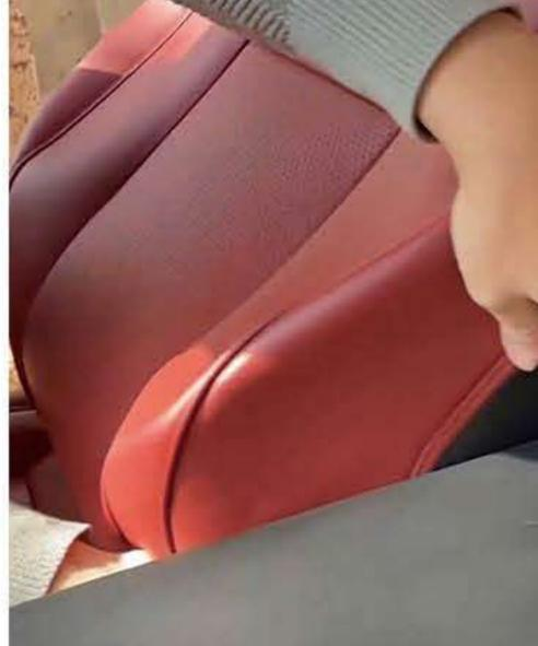
3. Adjust the seat cover and make it fits smoothly and seamlessly.Wrap the seat cover in place.
