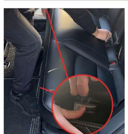
1. Pull the switch on the bottom of the seat. Remove socket. (Both left and right the rear seat. (Both left and right sides have one switch)
