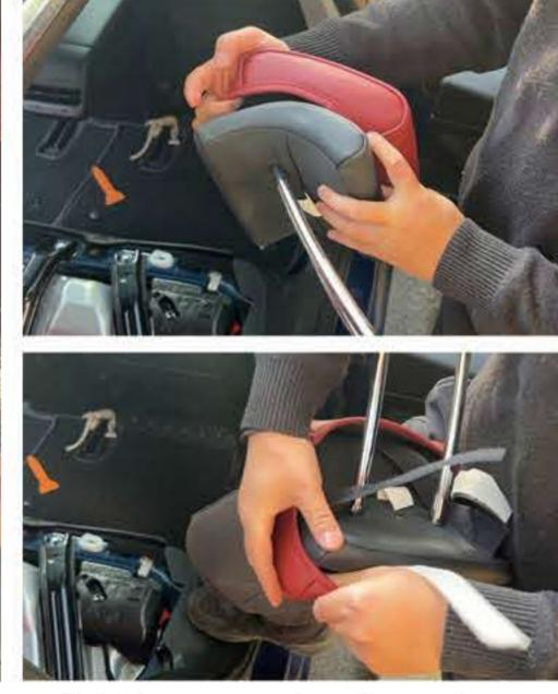
17. Put on the headrest cover is installed in place, back to the original place. affix the Velcro.
