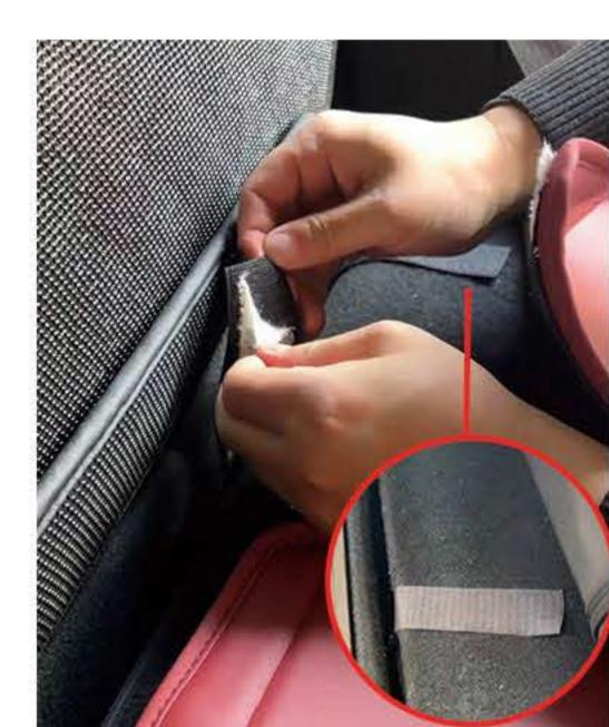
7. Pull out the Velcro, tear all the anti-stick cloth in the Velcro, and stick them to the back neatly.
