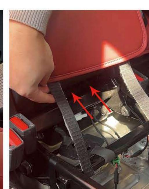
16. As before, the Velcro goes through the gap, tear the anti-stick cloth and sticks it to the back.
