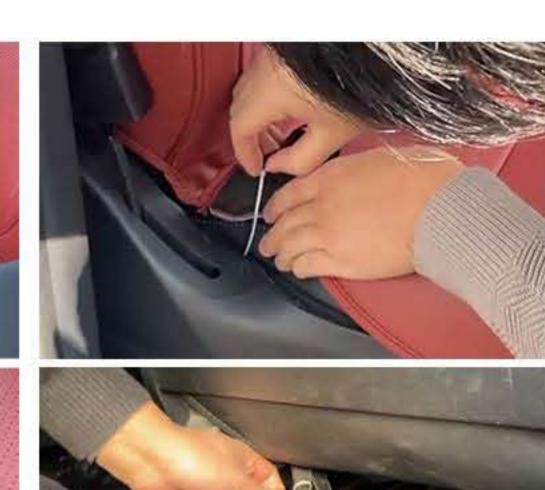
10. Insert the strip into the slit. And find the strip pull it out.(Same on the
