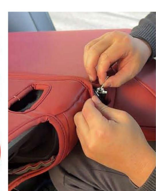
8. After the seat cover is installed in place, zip it up. anti-stick cloth on the
