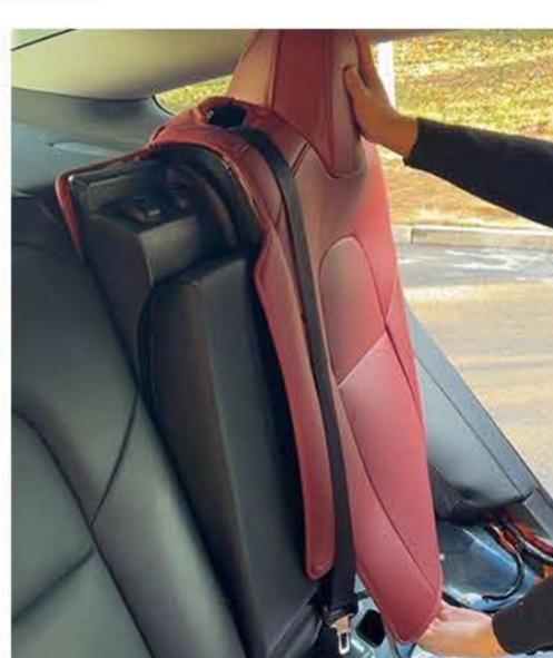
two parts. Unzip the seat the bottom. Go through cover and cover it on the the top of the metal bar. seat. Adjust the seat cover and take out the seatbelt.
