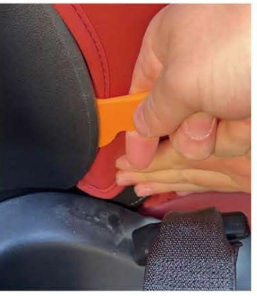
14. Use the tool to insert the side flap of the seat back cover into the gap.
