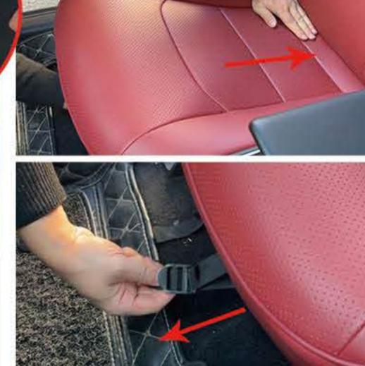
9. Press the position with the palm of your hand. Use your other hand to tighten the straps at the bottom.
