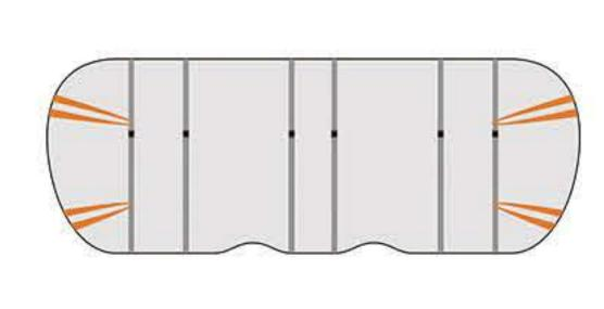
23. Installation of rear seat cushion cover, connect the bottom straps to each other.
