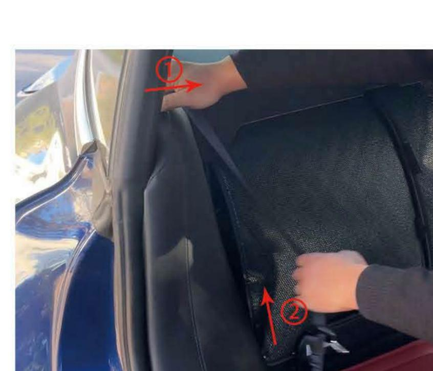
19. Removing the piece requires a bit of skill. Start by pushing it towards the inside of the car, then pull it towards the front of the car. Finally, lift it up from the bottom to successfully remove it.
