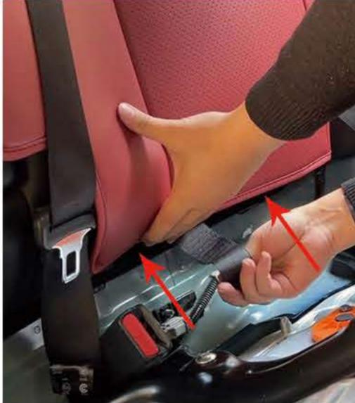
4. Split the seat back into 5. Pass the Velcro through 6. Pull the two seat covers
