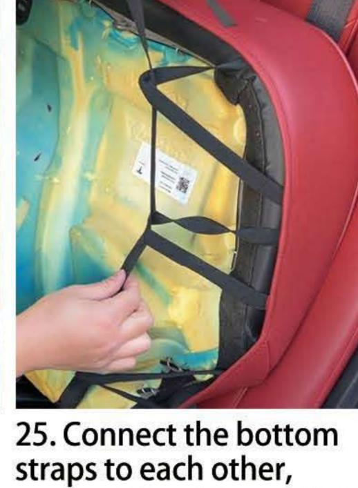
connect the side elastic belt by attach hooks or across through the side tapes.
